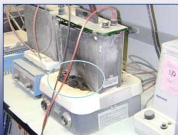
Heater/stir plate being used to stir was also accidentally turned on as hot plate!
